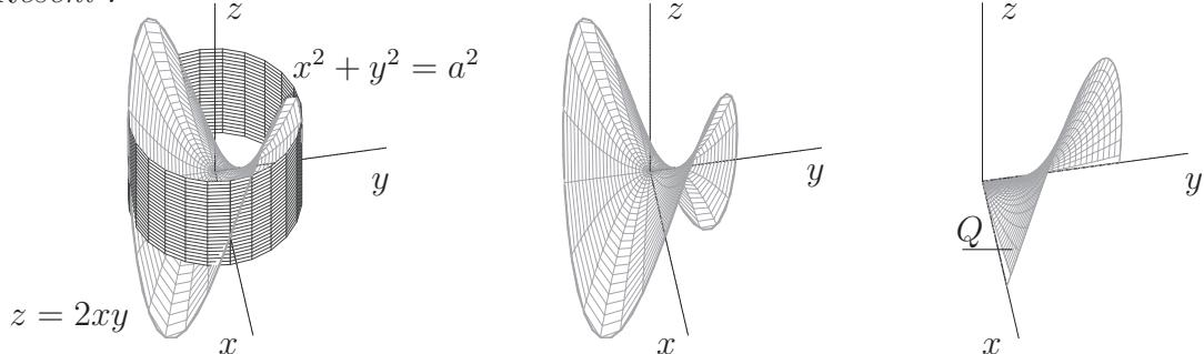
$$\begin{aligned} P(x, y) &= [x, y, 2xy], & B &= \{[x, y] \in \mathbb{E}_2; x^2 + y^2 \leq a^2\} \\ P_x &= (1, 0, 2y), & P_y &= (0, 1, 2x) \\ P_x \times P_y &= (-2y, -2x, 1), & \|P_x \times P_y\| &= \sqrt{4y^2 + 4x^2 + 1} \end{aligned}$$
