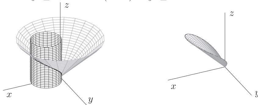
$$\begin{aligned} P(x, y) &= [x, y, \sqrt{x^2 + y^2}], & B &= \{[x, y] \in \mathbb{E}_2; (x - 1)^2 + y^2 \leq 1\} \\ P_x &= \left( 1, 0, \frac{x}{\sqrt{x^2 + y^2}} \right), & P_y &= \left( 0, 1, \frac{y}{\sqrt{x^2 + y^2}} \right) \\ P_x \times P_y &= \left( -\frac{x}{\sqrt{x^2 + y^2}}, -\frac{y}{\sqrt{x^2 + y^2}}, 1 \right), & \|P_x \times P_y\| &= \sqrt{\frac{x^2}{x^2 + y^2} + \frac{y^2}{x^2 + y^2} + 1} = \sqrt{2} \end{aligned}$$
